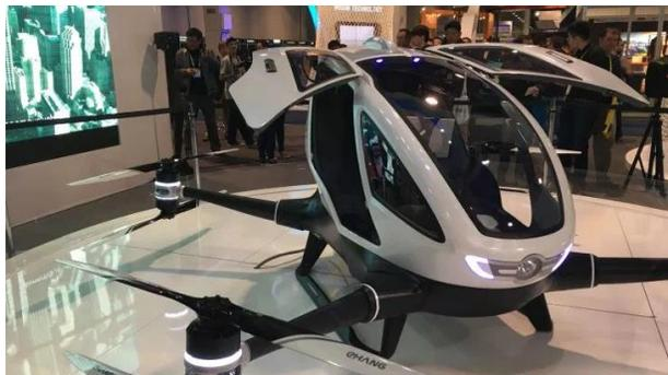
The Chinese drone manufacturer [Ehang](#) introduced the world’s first passenger drone, the [Ehang 184](#). With an ability to fly for 23 minutes at sea level, a passenger can set a flight plan and use only “Take off” and “Land” commands (with the help of a Microsoft Surface tablet mounted on the dashboard). With a 30-mile range, the applications are exciting. You could send the 184 out unmanned and return it with a person inside.
